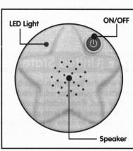
Press power button to turn the module on or off.
