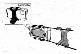
**B.** Attach case to the blaster rail. (If necessary, remove shields before attaching case to blaster rail.)
