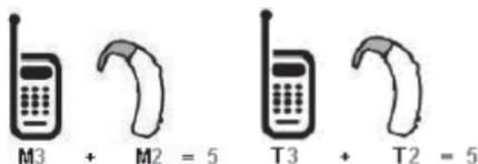
In the above example, if a hearing aid meets the M2 level rating and the wireless phone meets the M3 level rating, the sum of the two values equal M5. This should provide the hearing aid user with “normal usage” while using their hearing aid with the particular wireless phone.
