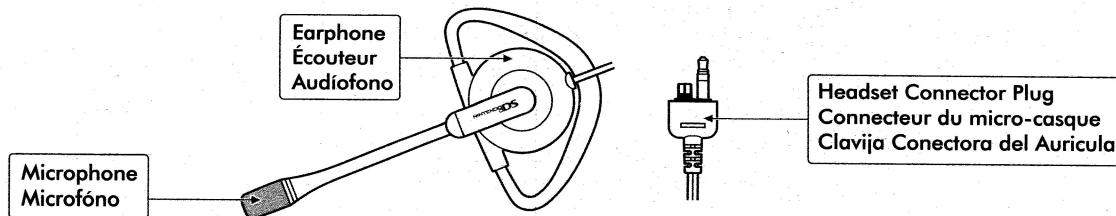
To install, insert the connector plug into the Headphone Connector on the front of the Nintendo DS or DS Lite.
