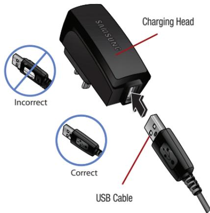
2. Insert the USB cable into the device's charger/ accessory jack.
