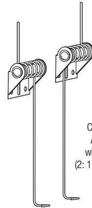
Cable Keeper Assemblies with Hardware (2: 1 Right + 1 Left)
